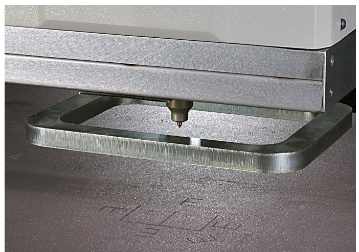
The PinStamp marker uses a hardened steel tip to mark text on plate
