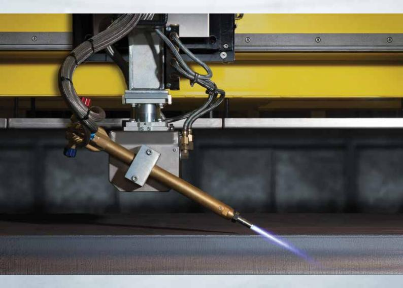
The ultimate oxy-fuel bevel system for complex cuts and thick materials.
