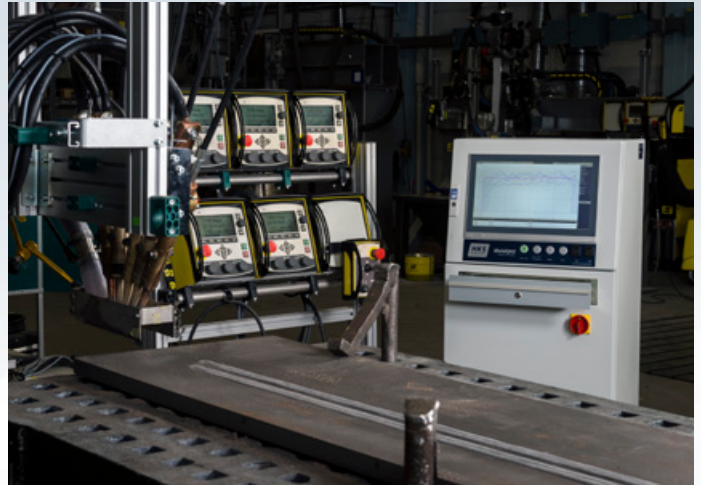
Multi-wire setup with PEK and WeldQAS
