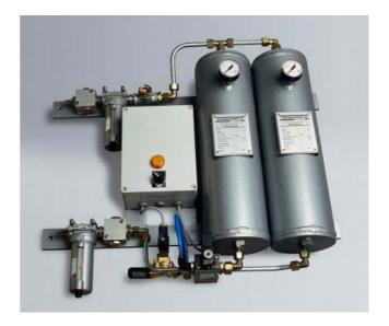
With ESAB's flux recovery system OPC or flux tank TPC 75, the air consumption is max 300 l/min. A compressed air system having dew point 0°C will give an increase of hydrogen in flux of 0.05% which is maximum for unspecified welding.
